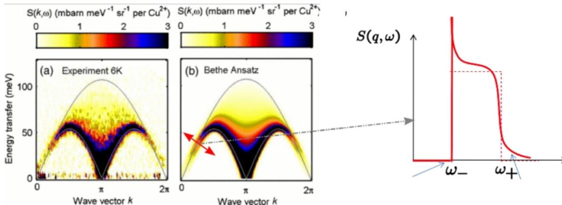
Left: Comparison between ABACUS and inelastic neutron scattering for  $KCuF_3$ . [PRL 111 137205].
